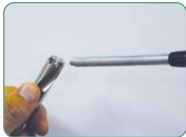
Make sure to clean the insert and insert seat.
