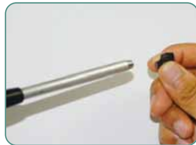
Make sure to clean the insert and insert seat.
